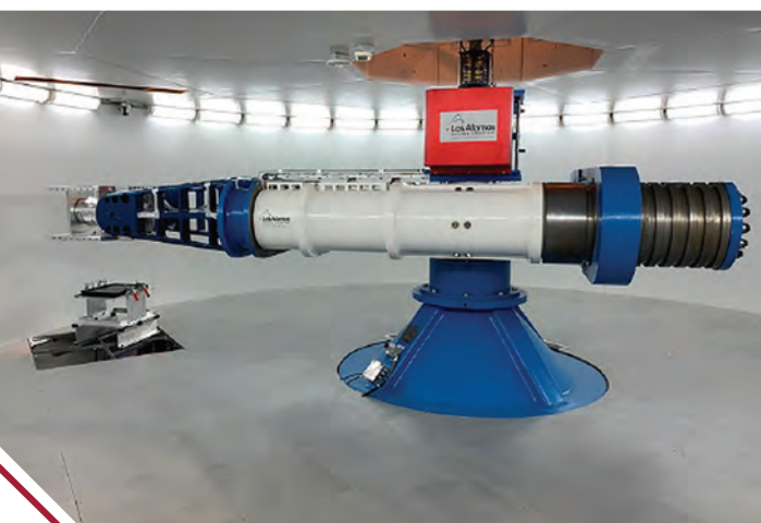
The Centrifuge Test Facility's flash X-ray system. Los Alamos National Laboratory.
