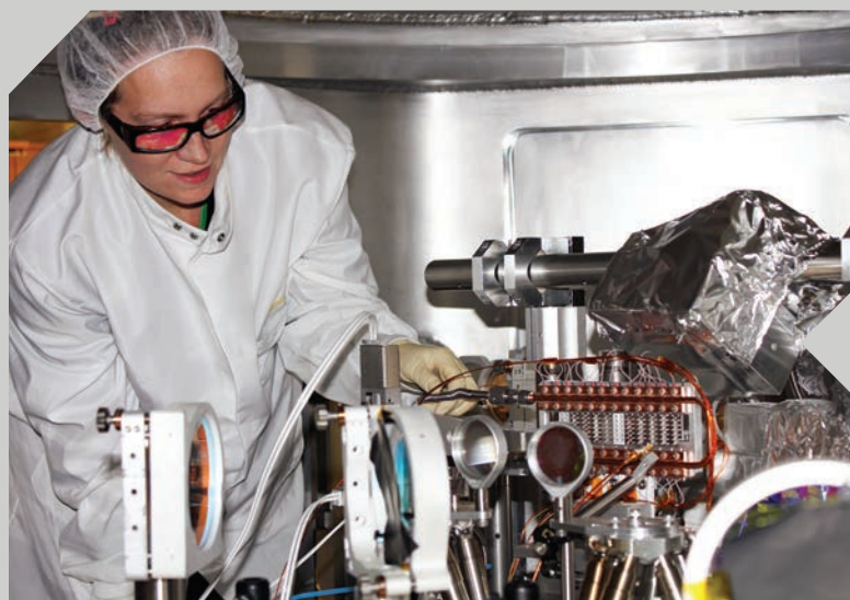
Arianna Gleason makes final adjustments to detector positions inside the Matter in Extreme Conditions target chamber at the SLAC Linear Accelerator Laboratory.
