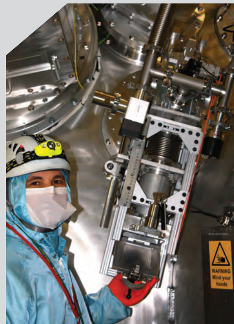
An engineer installs a spectrometer that measures samples' densities during experiments on the Orion laser.
