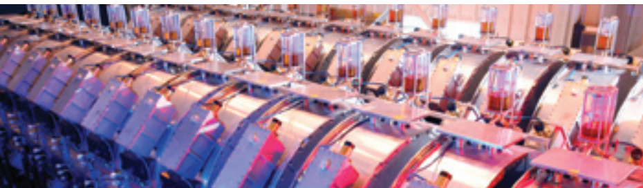
Circular aluminum structures create magnetic fields in DARHT's accelerator, focusing and steering a stream of electrons.
