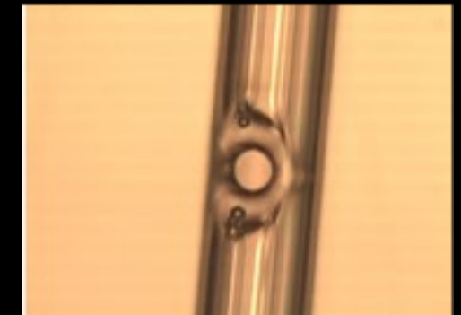
Laser machined gas inlets
