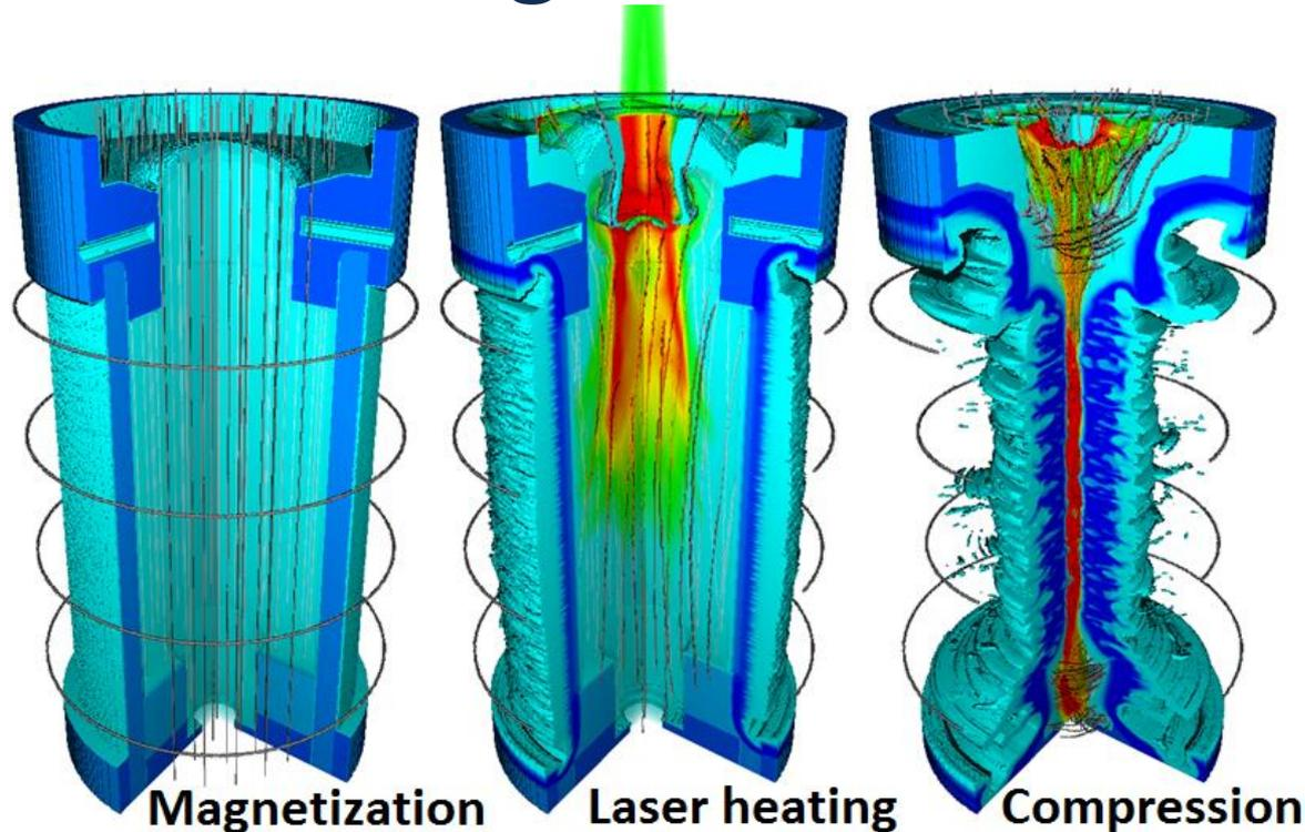
Magnetization and laser heating relax the implosion velocity, areal density, and convergence requirements of inertial confinement fusion
