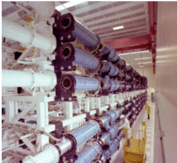
Shiva laser (1978) 20 beams 10,000 Joules
