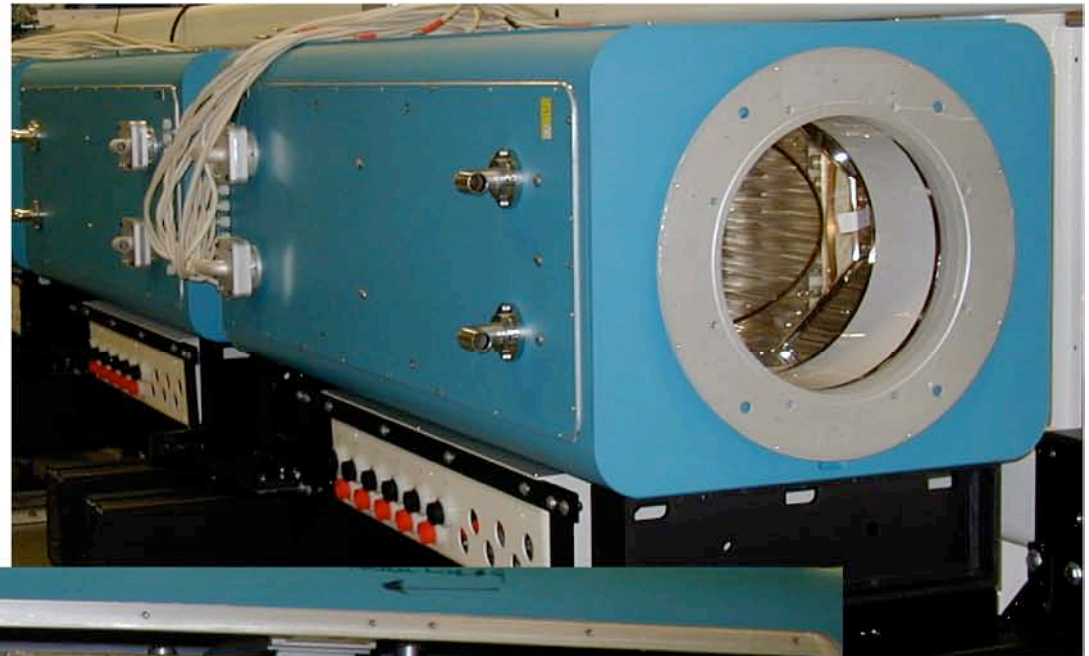
31 cm Disk amps from NOVA
