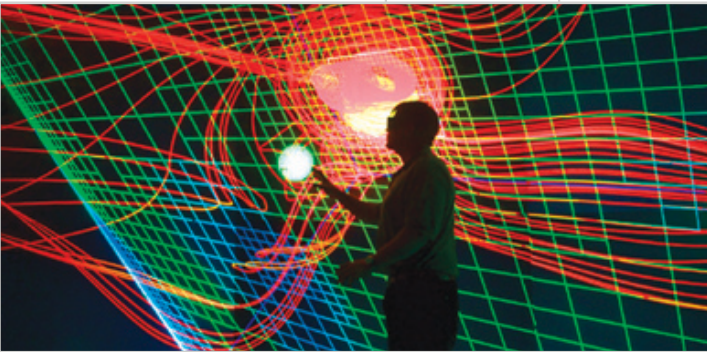
The Los Alamos National Laboratory CAVE uses 33 projectors to create a 43-million-pixel virtual reality environment. Researchers can simulate a problem, then walk through its visualization to detect trends, correlations, anomalies and unusual events.
