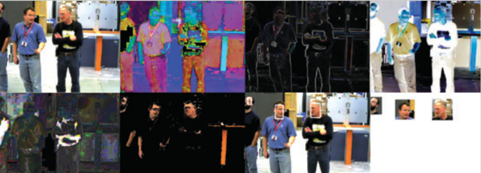
This montage shows the steps used to extract faces from video image data. Shown from the upper left to the upper right are the original frame, the RGB-to-HSI converted frame, the Sobel edge-detection filtered frame and an inverse color frame. The bottom row shows an RGB entropy frame, skin-colored pixel patches, the faces framed for easy visual identification and the final identified faces. These are added to the face database.
