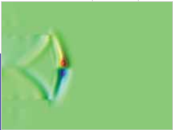
Beam 1: The bunch is just passing the junction where the pipe is attached to the cavity.
