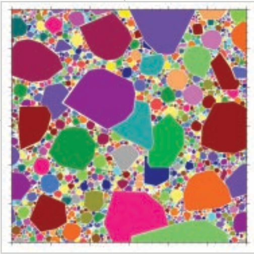
Synthetic photomicrograph of a computer-generated plastic-bonded explosive illustrating a bimodal grain-size distribution without defects. Each color represents a distinct crystal orientation. The plastic binder shows as a white outline around each grain. Slice is 0.3 x 0.3 mm.
