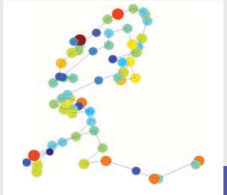
The same walk shown as coarse-grained chain of 64 beads, with each bead located at the center-of-mass of the corresponding 32-bead segment of the original 2048-bead chain. The colors (moving from blue to red) indicate the relative configurational energy of the bead, as determined by summing up the individual stiffness penalties of each segment.
