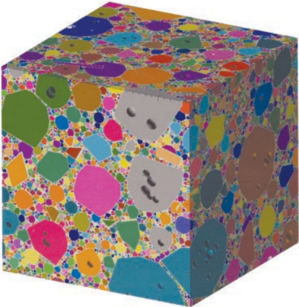
The computer-generated 0.3 mm cube contains approximately 0.1 million HMX grains with a bimodal grain-size distribution. Defects, shown as spherical voids, are present in the larger grains. Those that are intercepted by the surface of the cube appear as divots. Each color represents a distinct crystal orientation.
