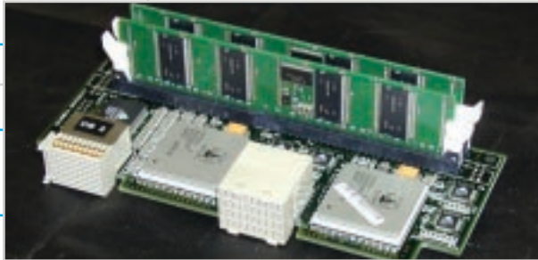
A QCDOC daughterboard with two ASIGs and two DDRIMMs. The cubic blocks are connectors.
