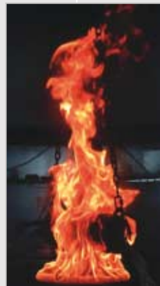
These images are photos taken from a high speed video (500 fps) as part of an experiment at the University of Utah. They are images of a burning pool (12 inch diameter) of Jet A fuel. The different frames are 80 ms apart. This experiment is an actual fire similar to the one illustrated by the simulation images on page 9.
