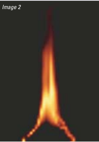
Both images are snapshots (one time frame) of a transient 3-D 1 meter heptane pool fire simulation completed at the University of Utah. These images show the soot volume fraction in the fire. Image 1 simulation uses traditional equilibrium calculations for chemistry. Image 2 uses the intrinsic lower dimensional manifold (ILDm) method for the chemistry calculation. ILDM is what Nguyen is working on as part of her dissertation.
