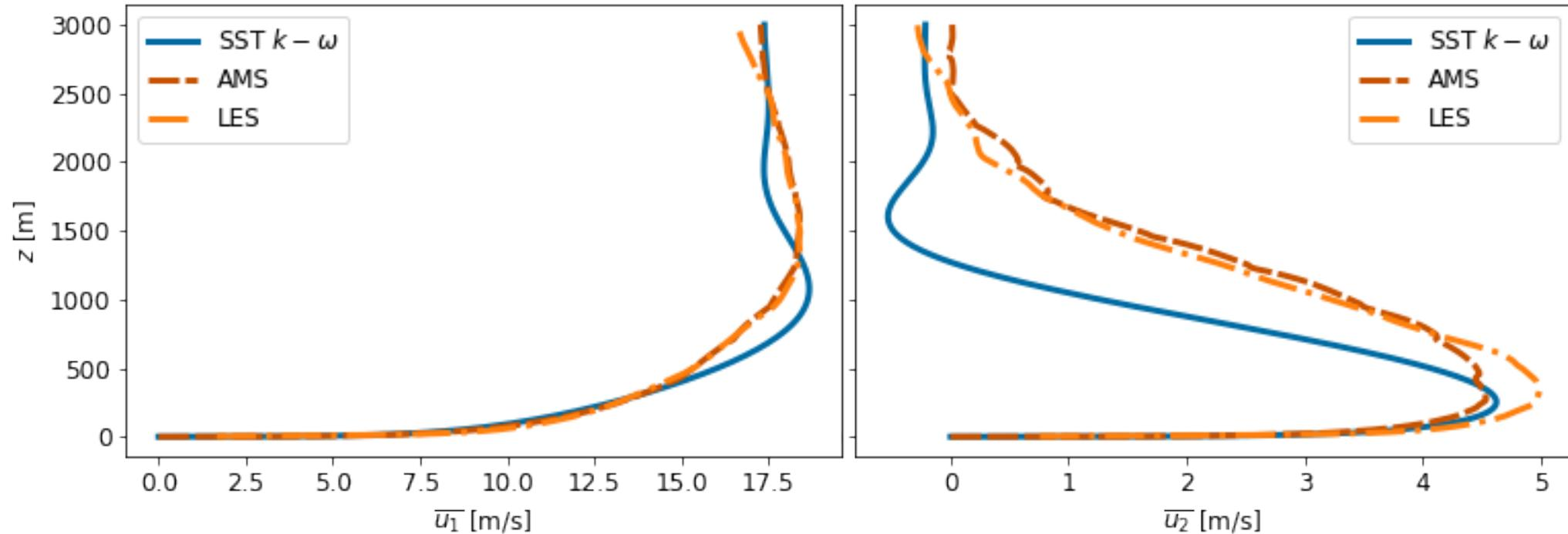
AMS with  $l_t$  and  $T_{l_t}^R$  matches LES well; better than SST does
