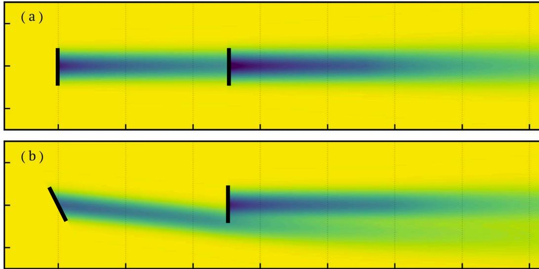
Find yaw angle for each turbine to maximize total power that wind farm produces
