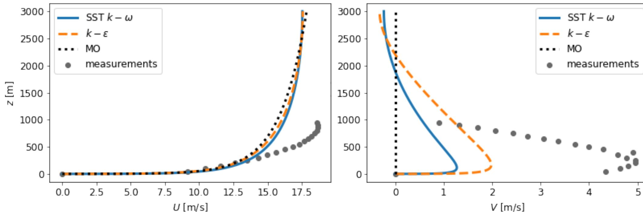
Measurements from Leipzig Field test [8]
