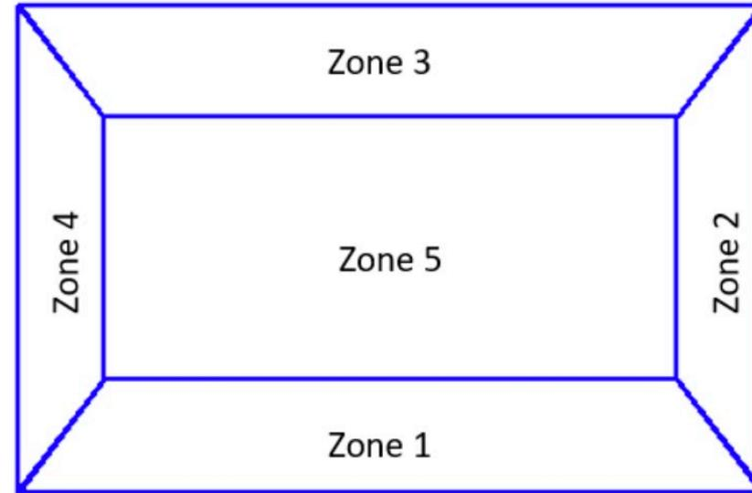
Keep temperature in each zone comfortable while minimizing cost by setting central cooling and fan power for each zone
