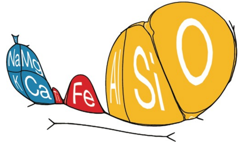
Periodic table scaled by abundance of elements in earth's crust, by weight
