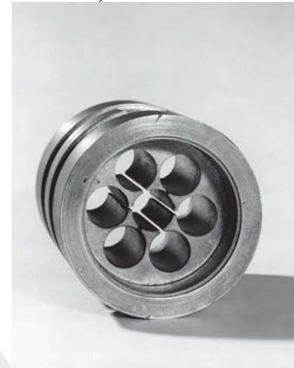
Figure 2: Cavity magnetron by Mr. John Cummings CC-BY-SA 2.0
