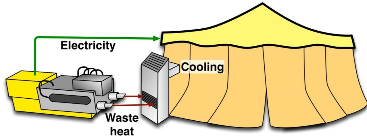
Fully thermally activated air-conditioning in remote locations
