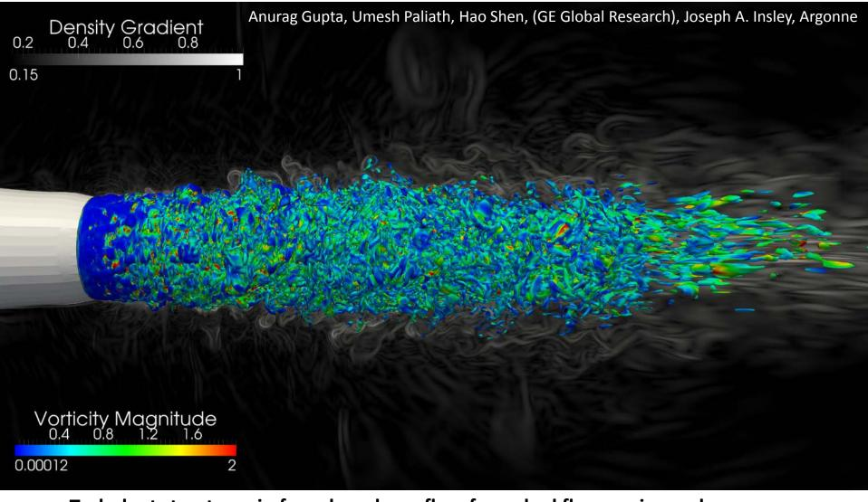
Turbulent structures in free shear layer flow from dual flow conic nozzle
