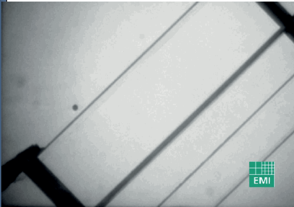
Hypervelocity impact test of multi-layer micrometeorite shield
